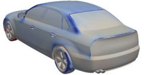
Fig. 1a Overall drag sensitivity to normal displacement of the surface based on the steady-state (SS) adjoint.
