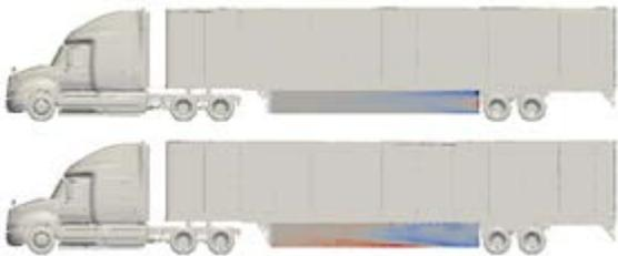
Fig. 6a Drag sensitivities on the side-skirts for a tractor-trailer for SS (top) and QT (bottom) solutions.
