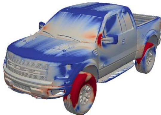
Fig. 4 Drag sensitivities for the pickup truck using the QT solver
