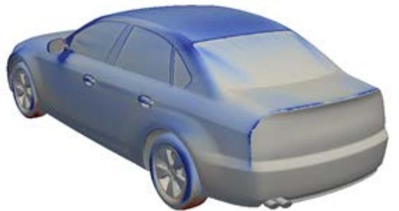
Fig. 1b Overall drag sensitivity to normal displacement of the surface based on the quasi-transient (QT) adjoint.
