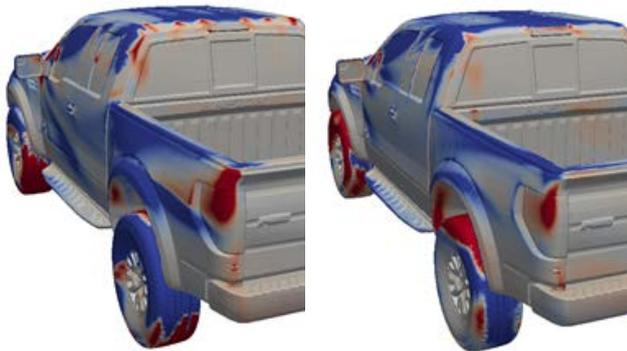
Fig. 2 Drag sensitivities for the pickup truck using the SS solver (left) and QT solver (right).
