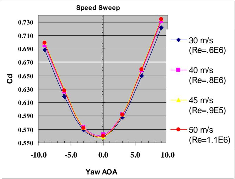
Figure 3 –  $C_d$  vs Yaw at various test speeds
