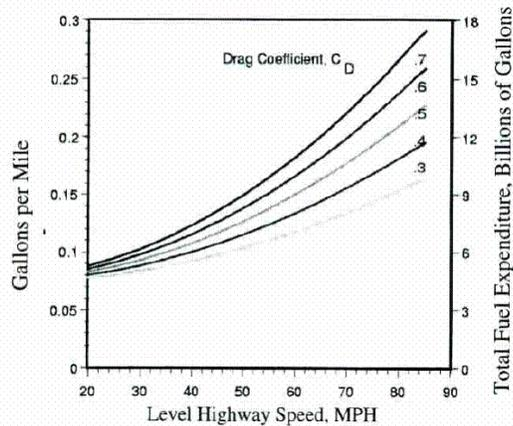
Figure 2 – Fuel consumption for typical Class 8 Truck [10]
