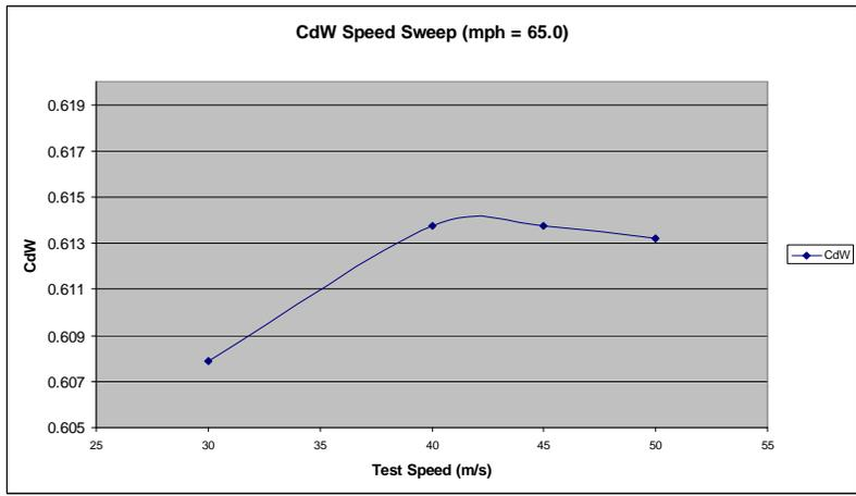
Figure 4 - Wind averaged drag vs Test Speed
