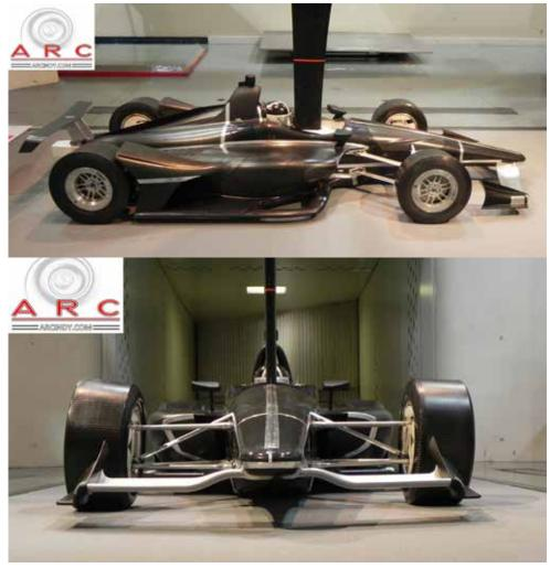
The 50 per cent scale UAK18 model in the ARC Wind Tunnel during aerodynamic testing. Courtesy of ARC
