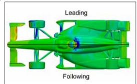
Figure 8: This is the same comparison of the surface pressures acting on the 2017 Honda bodykit, viewed from above the car
