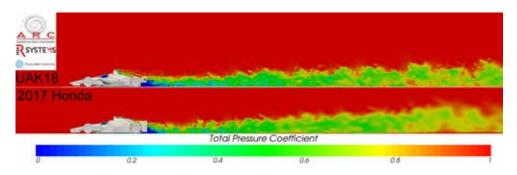
Figure 2: Comparison of total pressure coefficient for the single-car case along the centreline of each car, seen in profile. The Honda wake grew taller as it travelled downstream whereas the UAK18 wake maintained a relatively consistent height
