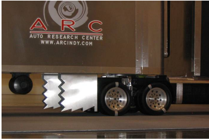
Figure 12: Development wheel splitter device mounted behind rear truck wheels.
