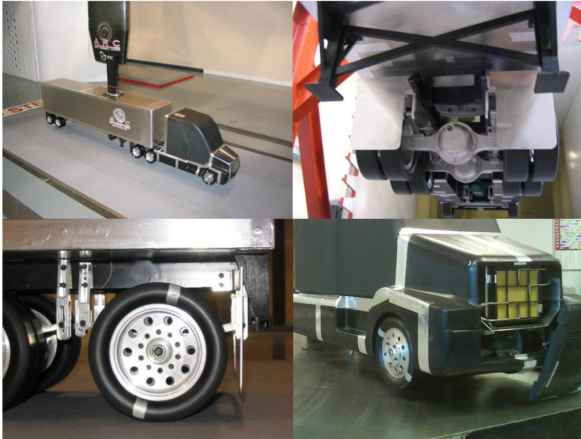
Figure 4 – ARC detailed undercarriage featuring accurate rolling wheels and internal radiator/engine flows
